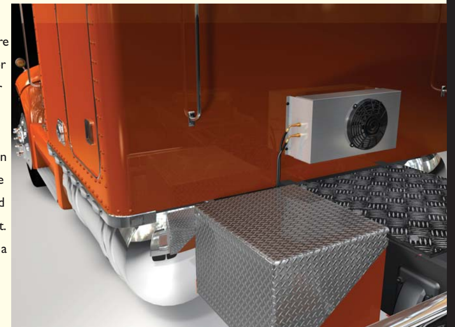
Split system outside condensing unit.
